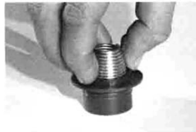
Make sure the support flange also is up, toward the throat of the spring. Check to be sure the new spring is seated firmly and centered in its support. Locate the polyethylene sleeve and rubber damper ass'y. Slide the polyethylene sleeve, narrow end up, onto the suspension levelling stem.
