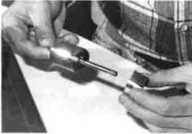
Find the weight assembly collar and begin to thread the carrier rod into the hole. Do not thread the rod in all the way.
