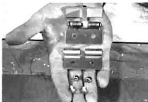
4) Take the hinges 1 at a time and place them against the outside of the dust cover with the T-shaped part of the hinge facing away from the cover. Position the loose metal plate on the inside of the cover and align the holes so that the screws may be inserted. Push the screws through from the inside of the cover and hand tighten the cap nuts.
