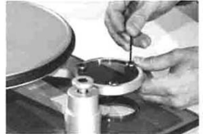
Refer to the instructions supplied with your tonearm to locate the correct distance from the spindle to the drilling center, and the size of the hole to be drilled. Check to see that you have adequate clearance behind the tonearm to clear the dust cover when it is closed. Rotate the tonearm board to obtain the most convenient positioning of the arm relative to the arm board screws. Using a sharp tool, mark the arm board for drilling.
