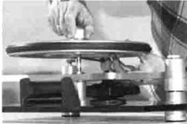
When you feel the spindle tip touch bottom (the thrust pad), position the drive belt around the motor pulley.
