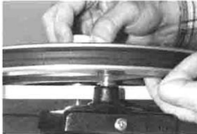
Slowly rotate the platter 1 or 2 times by hand to seat the drive belt properly. Adjust the suspension height so that the top edge of the belt rides approximately in the middle of the platter's inner rim.
