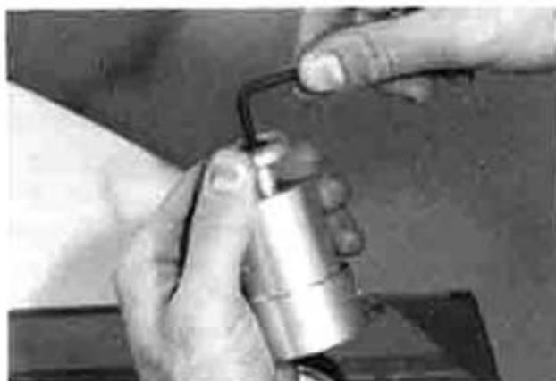
Set aside the top screw and levelling knob. Lift off the suspension housing; the spring is now easily accessible.
