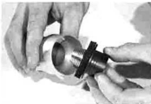
Slide the suspension levelling stem through the bottom end of the spring until it seats on the upper spring sleeve.
