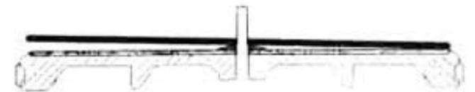
3) Place the coupling disc over the spindle and screw it down until it just touches the record label. This brings the record into contact with the mat only at the edge, or not at all.
