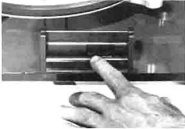
2) Press the button just to the right of the On / Off button to select 33 or 45 rpm. The speed you have selected is indicated by 1 of 2 LED's at the right side of the switch assembly.
