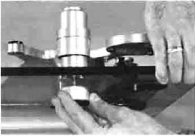
Only rough levelling is required now; precise levelling occurs after the turntable is moved to its final position. You can use a carpenter's spirit level to do this job.
