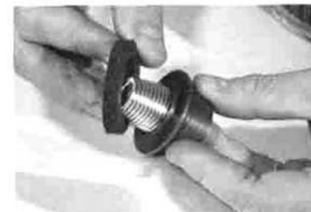
Slide this new spring assembly (spring, support and sponge rubber ring) into the suspension housing.
