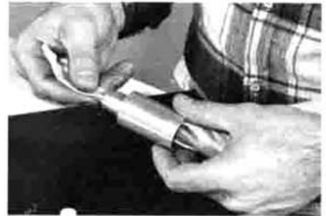
Visually inspect the bushings before reinstalling the bearing to see that they are completely clean and unmarred. Reposition the thrust pad in the baseplate cup. Install the brass baseplate in the bearing housing, making sure that the 3 screws are firmly in place. Return the bearing assembly to the subchassis. Install and tighten the 3 long screws. Since this system is self-aligning, no adjustment is necessary.
