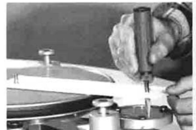
You may wish to scribe a reference mark across the outer edge of the arm board and inner edge of the subchassis to facilitate realignment after drilling.
