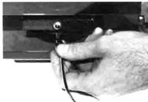
2) Keep the transformer / power supply away from any signal-carrying wires and as far away from the turntable as conveniently possible in order to avoid hum pickup.
